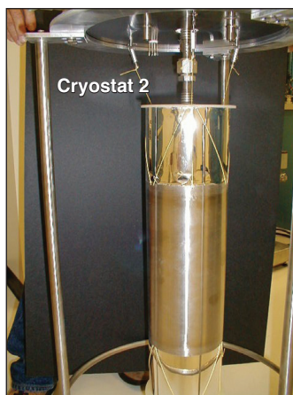
Figure 2. View of Cryostat-2 showing the cold-mass assembly mounted on a workstand.
